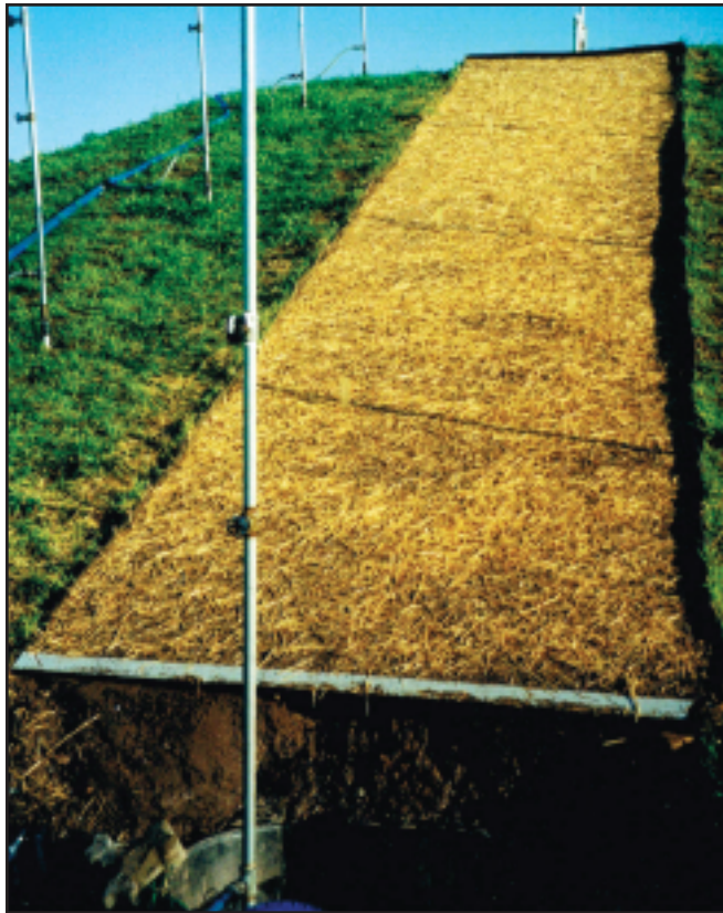
Blown straw (on left) and RECP (right) during testing.
